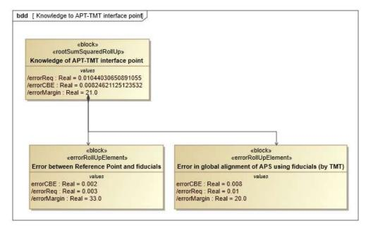
Figure 24 Alignment Error Budget
