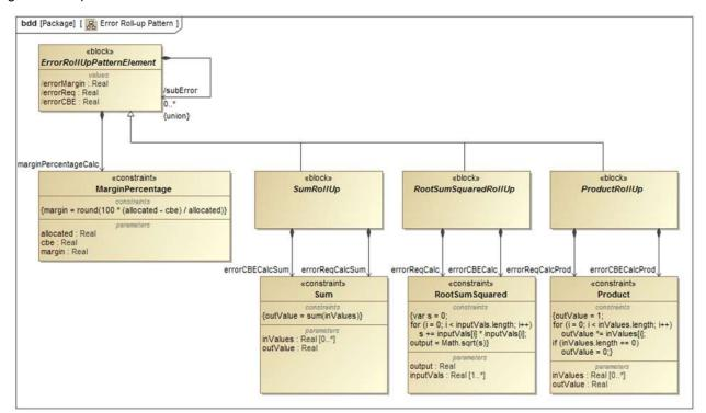
Figure 20 Different types of Roll-ups
