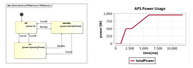
Figure 9. Peak power consumption analysis: (a) general pattern used and (b) result of executing analysis.
