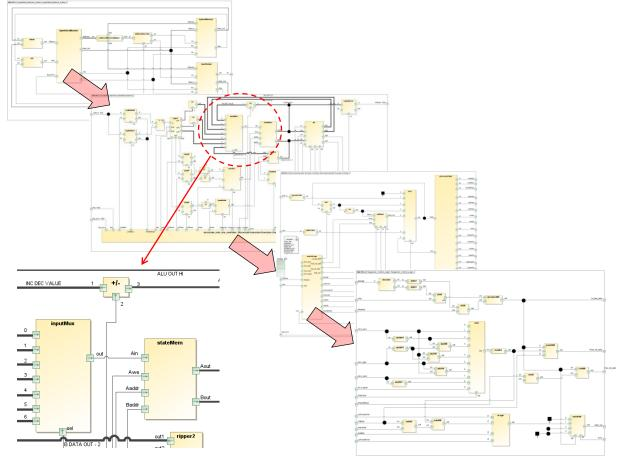
Figure 4: System decomposition is an integral part of the unified and consistent SysML model as opposed to a set of isolated drawings. The figure shows successive decomposition of components (top left to bottom right).
