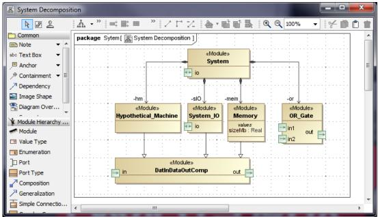
Figure 11: Module Hierarchy Diagram (MHD) showing the decomposition of an example System module
