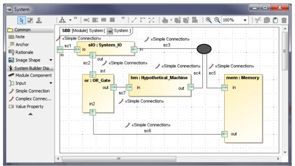
Figure 12: System Builder Diagram (SBD) showing the connections between ports of module components in the context of the example System module.
