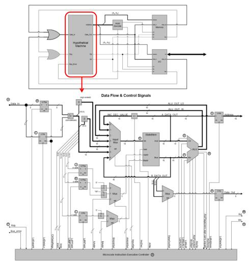
Figure 2: Drawings of an electronic system created by the system designer. The internal structure of the Hypothetical Machine sub-system (top) is shown (bottom).
