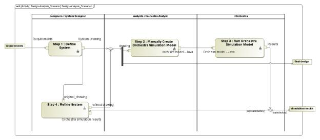
Figure 1: Document-based systems engineering of electronic systems before Maestro
